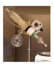
filtrate in a dry, pre-tared, 25-ml roundbottom flask. Evaporate off the solvent using a rota-vap. Weigh the flask with the product. Calculate the crude % yield. Scrape out the crude phenacetin and determine its melting point.
